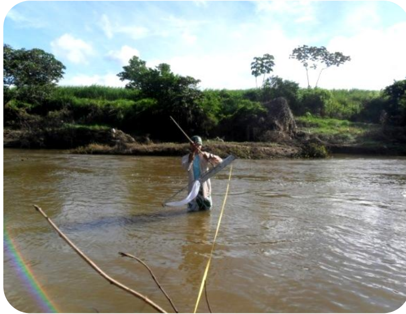
Figures 9. Bedload sampling with the sampler US BLH – 84 model.
