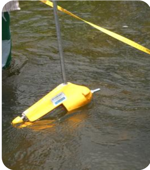
Figure 7. Suspended sediment sampling (sampler - US DH-48) in Capibaribe River.
